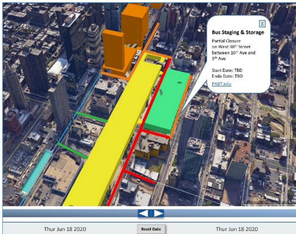
Figure D: Still frame example of 4D VDC content and progress with adjacent actual buildings and roadways, blocking of other theoretical buildings, with roadway impacts. Source: PMA Consultants, LLC., Port Authority of New York and New Jersey, Bus Terminal Design Competition
