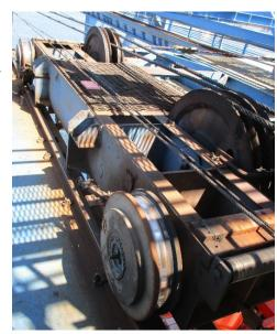
Photo above shows crane hoist trolley, trolley wheels, and trolley rail.
