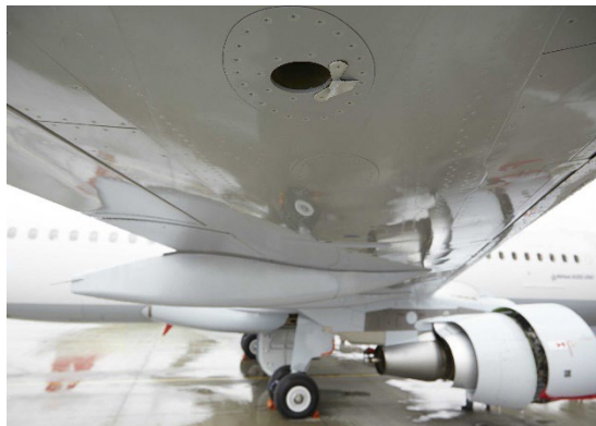
Image of Vortex Generator Device by Port on Wing.
