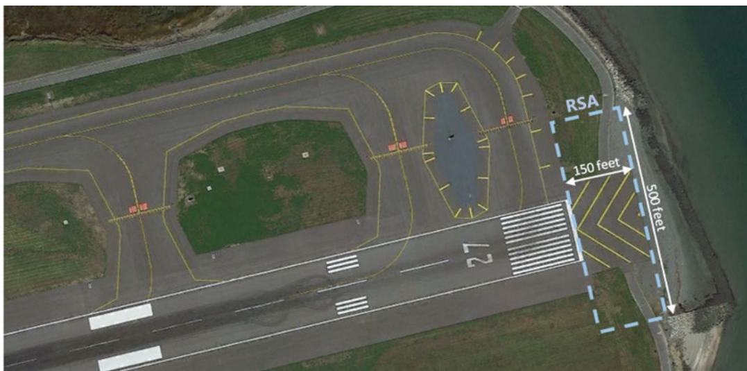
Figure ES-2 Runway 27 End - Existing Runway Safety Area
