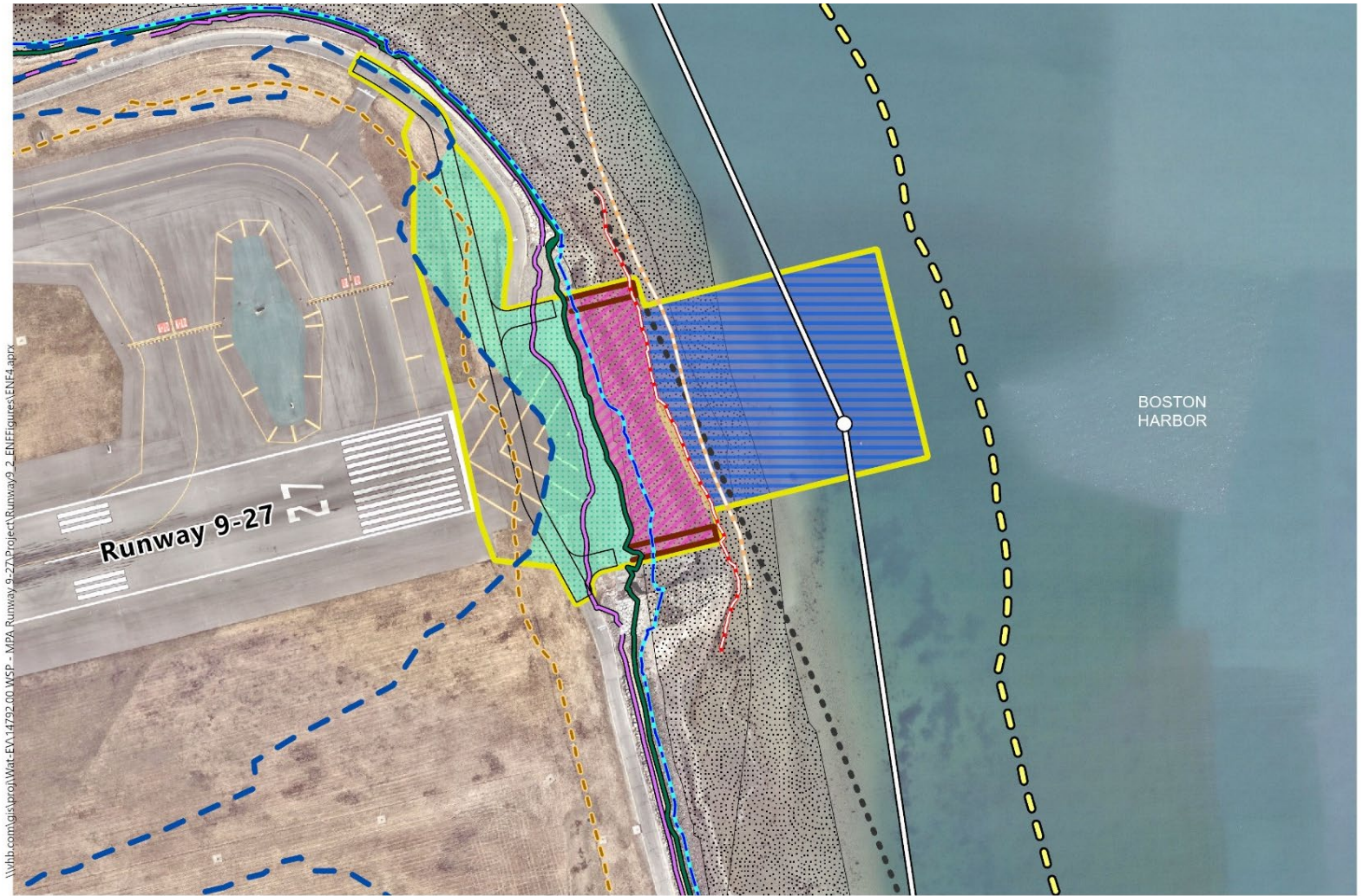
Figure E.2-7: Environmental Resource Areas Runway 27 End RSA Improvements Project Proposed Project Site Mean High Water Line Land Subject to Tidal Action Existing Airport Security Buoy (To Be Relocated) Proposed Emergency Egress Ramps Mean Low Water Coastal Beach Logan Airport 250-Foot Inner Security Zone Proposed Realigned Airport Perimeter Road Mean Lower Low Water Line Land Subject to Coastal Storm Flowage Legislated Logan Airport 500-Foot Security Zone Special Flood Hazard Area (100-Year Flood) Annual High Tide Line Land Under the Ocean Massachusetts Harbor Line (Approximated per Chapter 733 Acts of 1966) Coastal Bank Line 100-ft Coastal Beach Buffer Land Containing Shellfish Sources: WSP, VHB, NOAA 2021, FIRM Panel Number 25025C0101J, Effective Date 3/16/2016, Nearmap Imagery March 2022 Massachusetts Bureau of Geographic Information, MassGIS Data: Shellfish Suitability Areas, May 2011.
