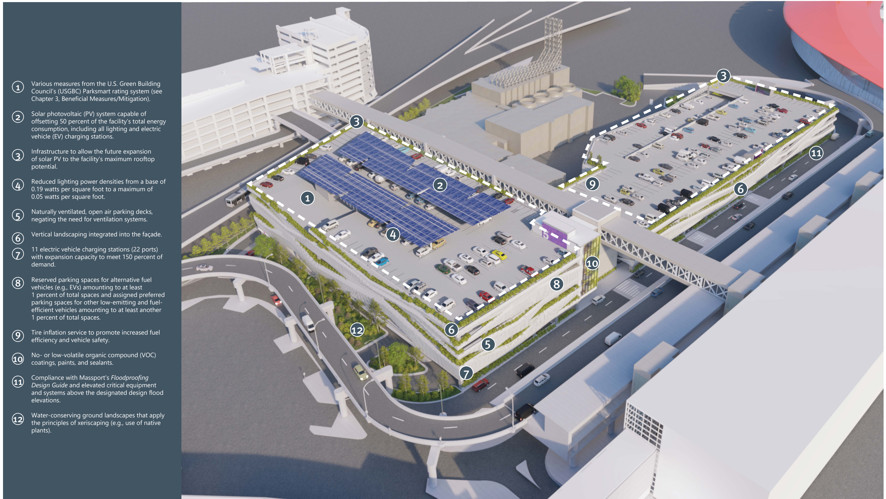
FIGURE 1-3 New Garage in Front of Terminal E, Proposed Massing and Major Sustainability Enhancements
