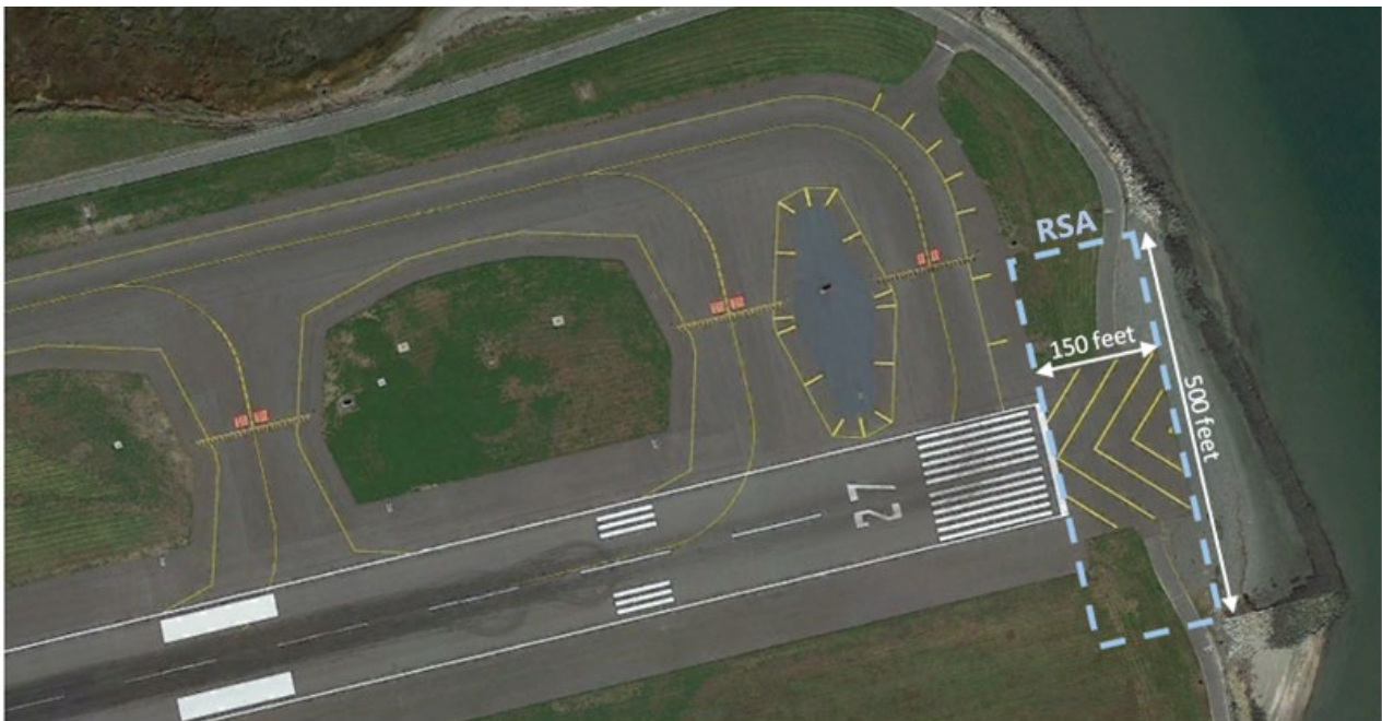
Figure ES-2 Runway 27 End - Existing Runway Safety Area
