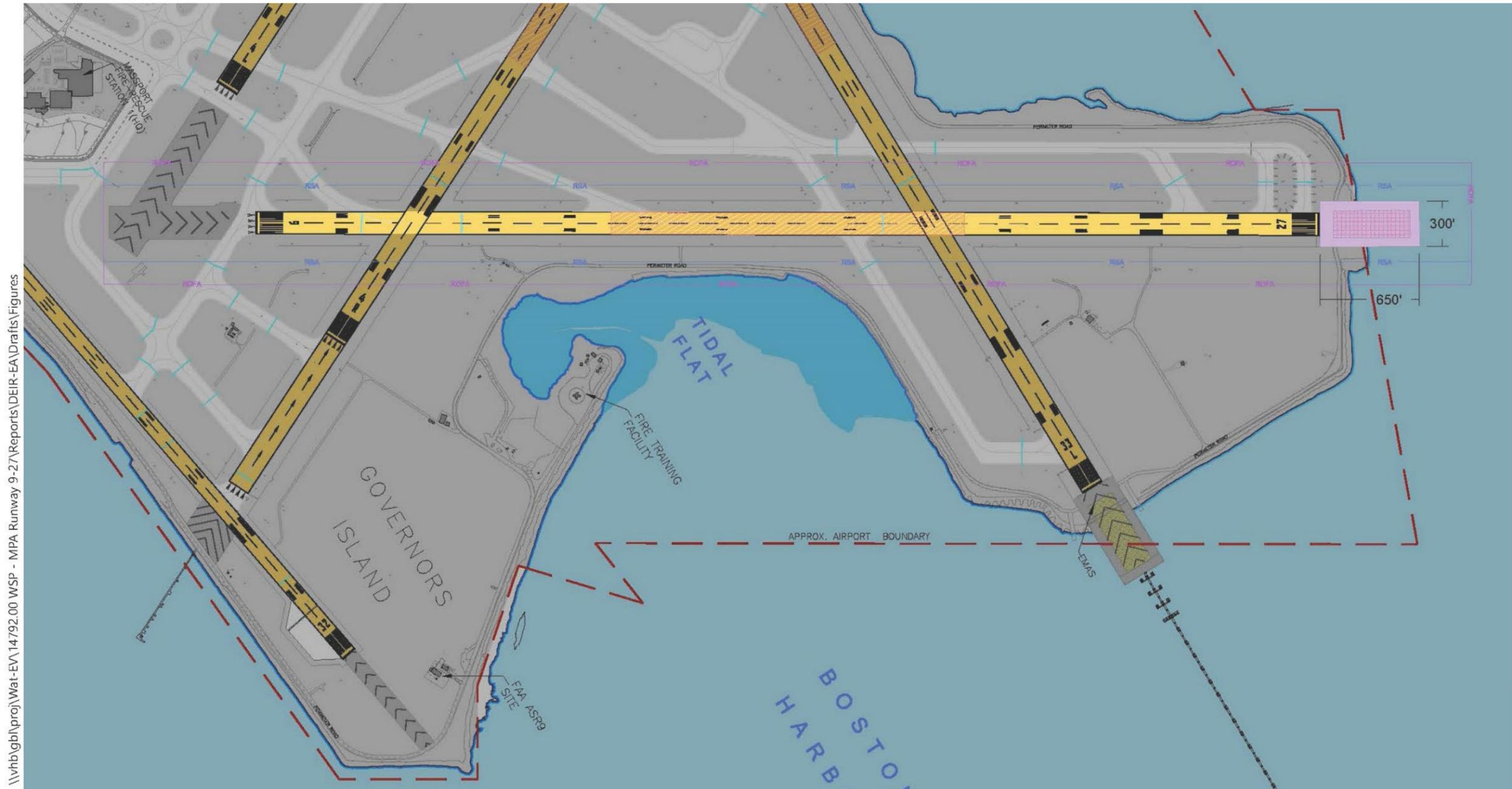
**Figure 2-8: Alternative 4B—EMAS on 306-Foot-Wide Deck (Proposed Action)**
