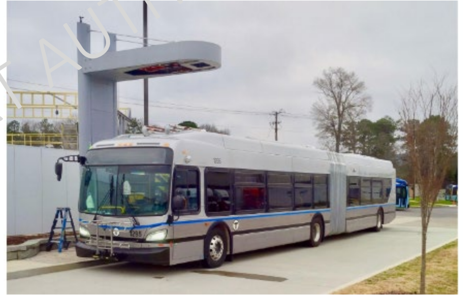
MBTA Silver Line Battery Electric Bus (BEB) with demonstration of en-route charging
