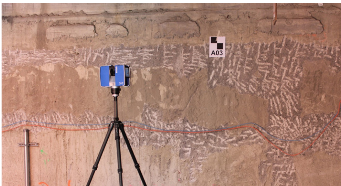
Figure 17: Temporary scanning target placed along slurry wall for concrete tolerance laser scan
