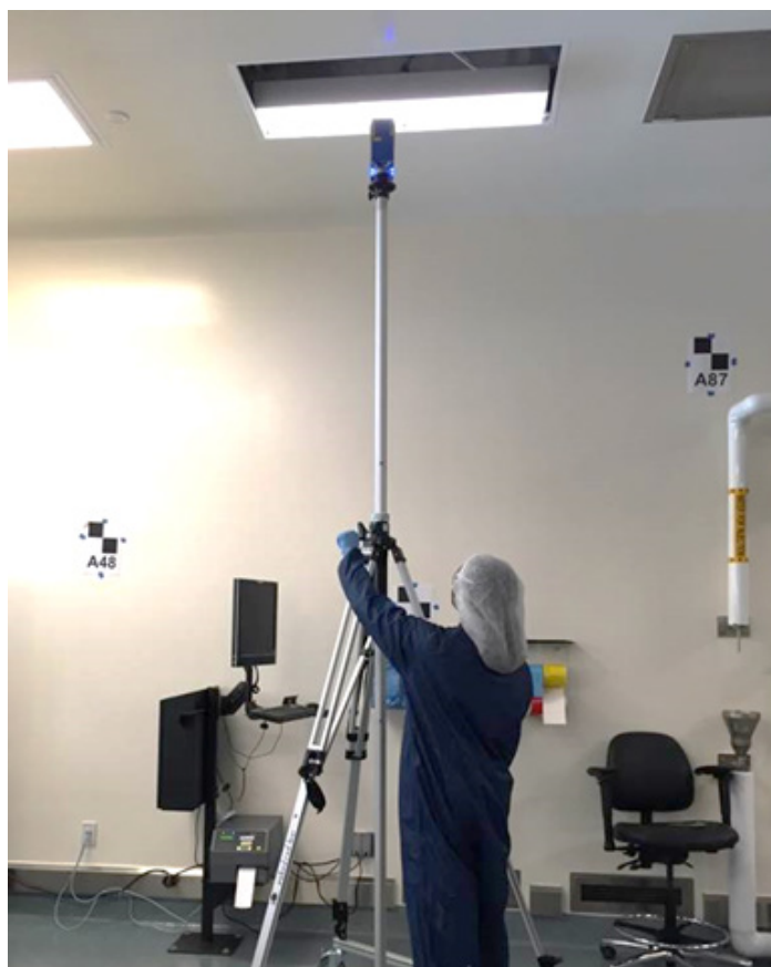
Figure 19: Laser scanning of above ceiling space accomplished with telescoping tripods. Targets distributed around above ceiling MEP
