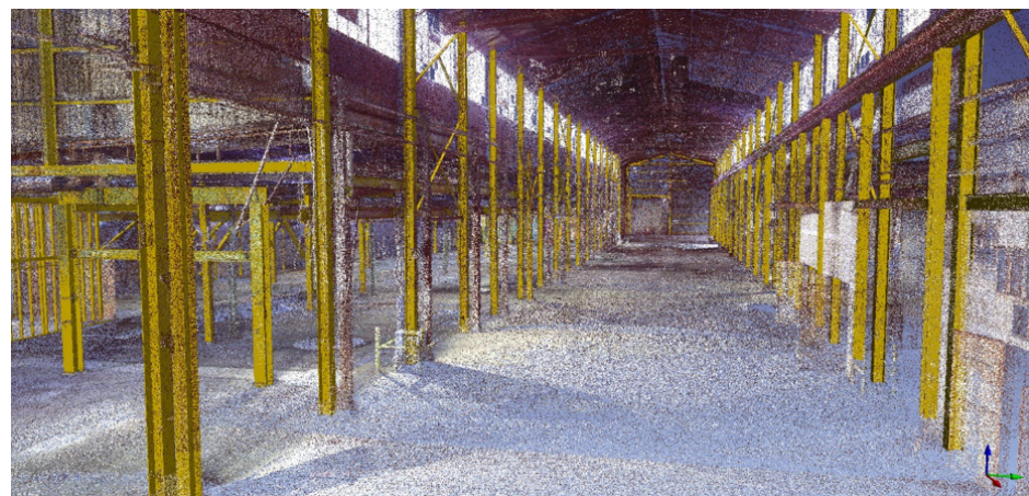
Figure 10: Point Cloud As-Built Verification against BIM
