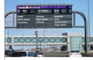
resolution refers to the number of pixels in in a given area. Pixel pitch is the distance he center of an LED pixel to the center of the next LED pixel and it is measured in eters. Resolution is measured in pixel pitch for LED signs. Lower resolutions create larger ters which are viewable at farther distances, while higher resolutions allow for shaper cs. The tighter the pixel pitch the more costly the sign, therefore finding the balance is
