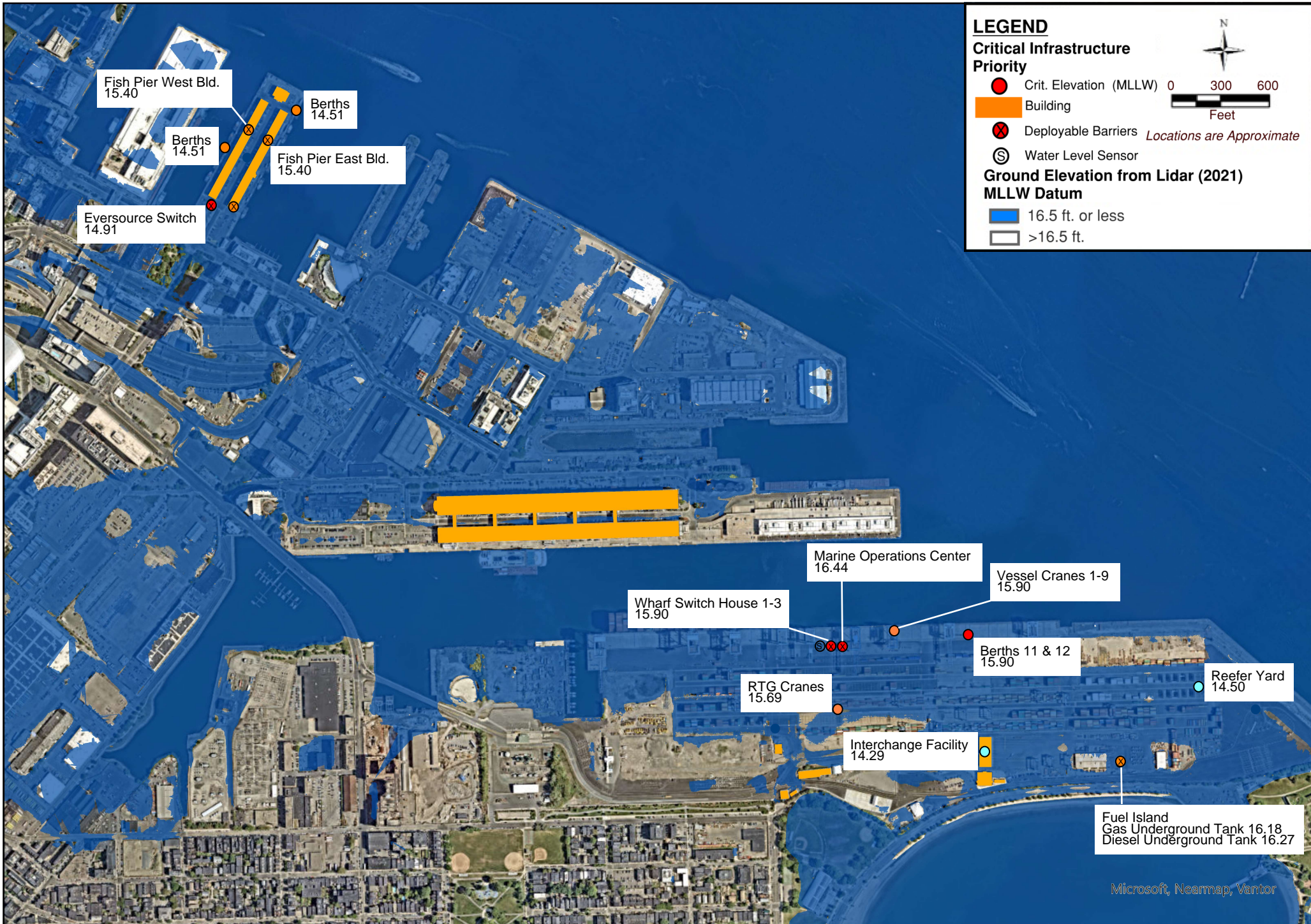
Figure 3 - Maritime Facilities at Risk of Flooding below 16.5 MLLW
