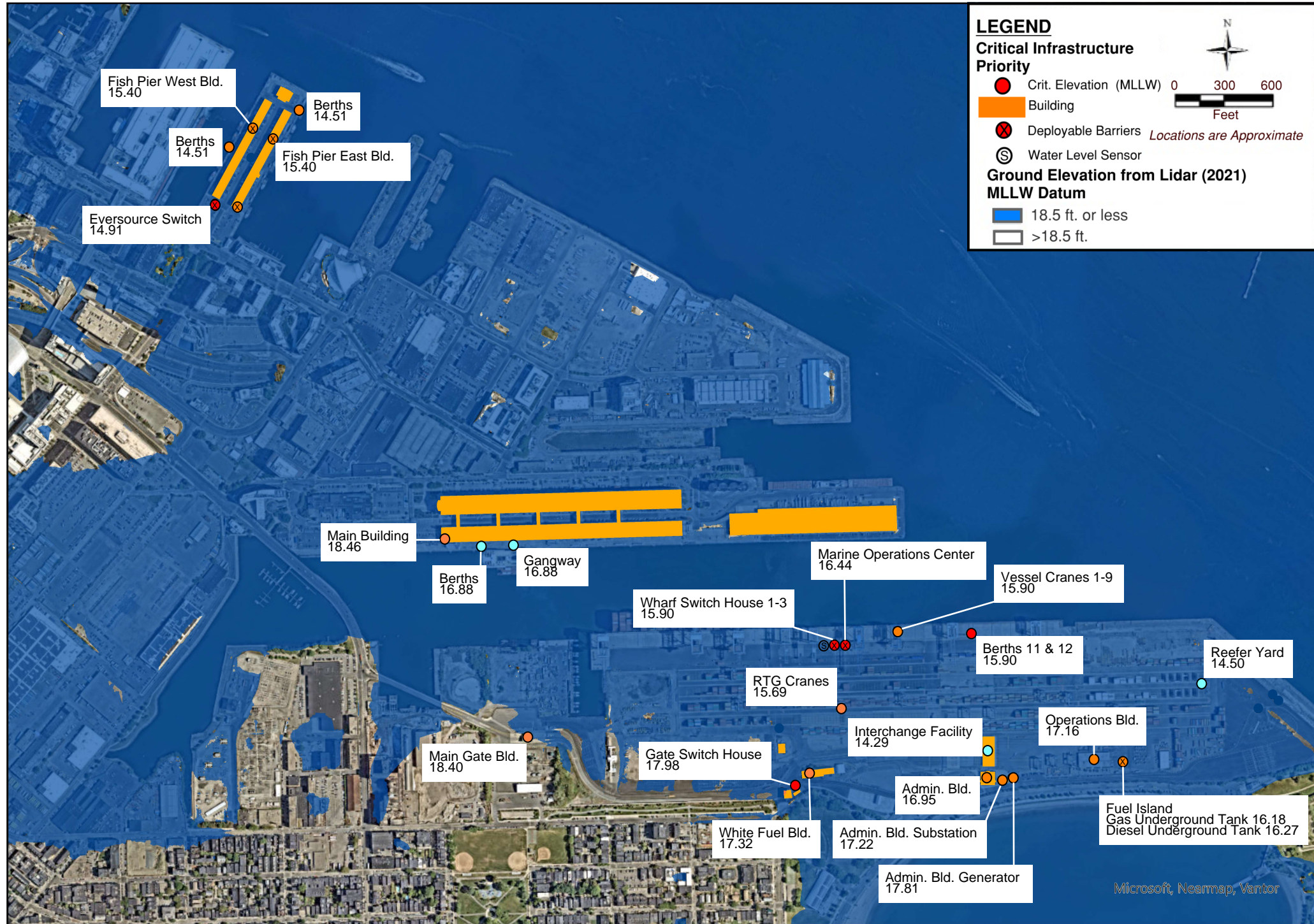
Figure 5 - Maritime Facilities at Risk of Flooding below 18.5 MLLW
