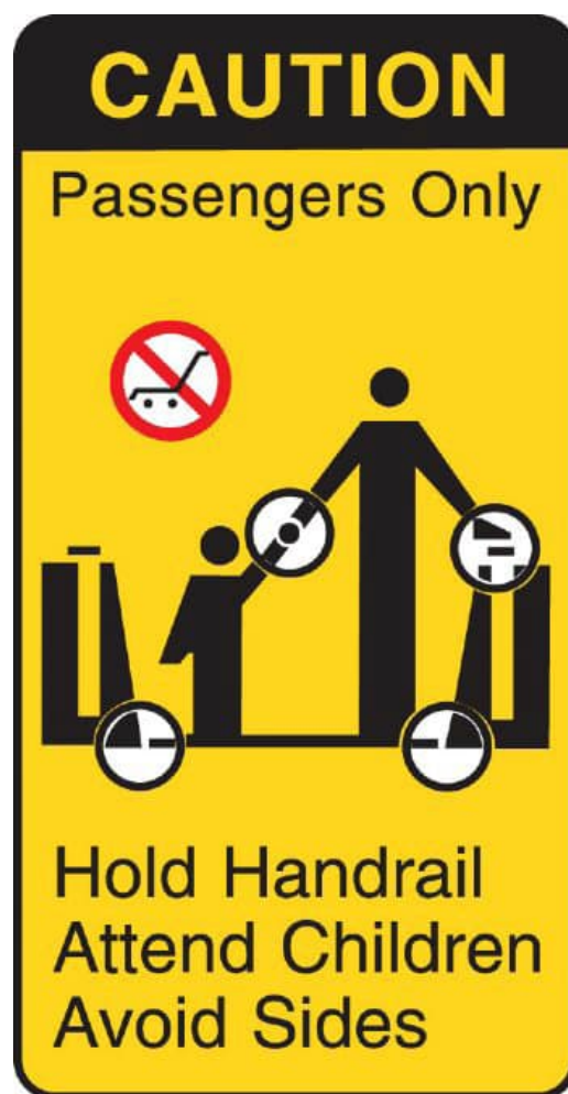
Figure 2: Required Caution Sign (6.1.6.9.1) (sign size, minimum 4"W x 7.75"H)
