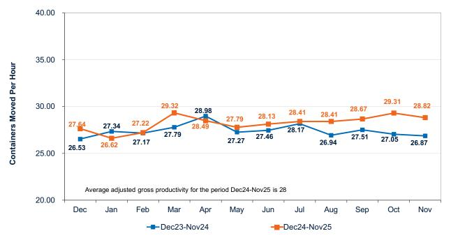
Productivity is determined by averaging the number of containers lifted per hour per crane during the time vessel operations are underway. Vessel operation time is determined by the time the vessel is at berth minus delays.
