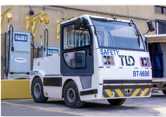
eGSE at airside charging port
