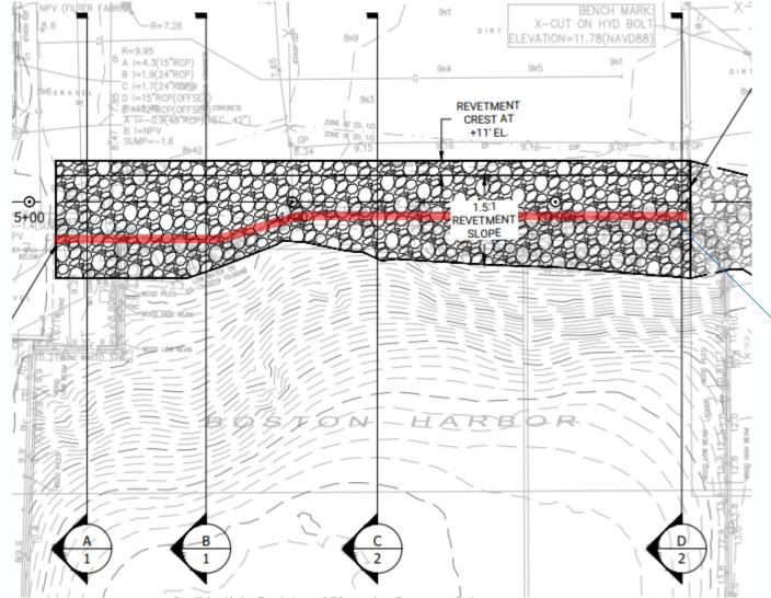
PLAN PROPOSED SLOPED STONE REVETMENT
