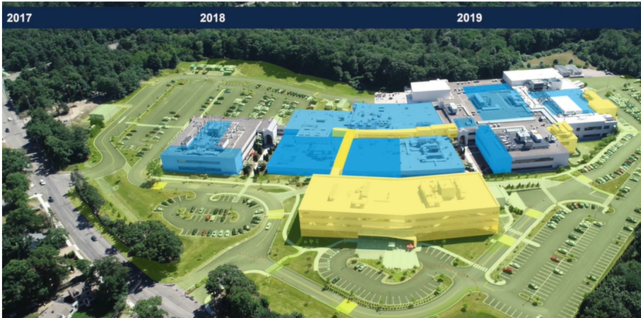
Figure A: Example of 4D animation (still frame image shown) making general assumptions of building timing and shape. Source: PMA Consultants, LLC., Columbia Construction Co.
