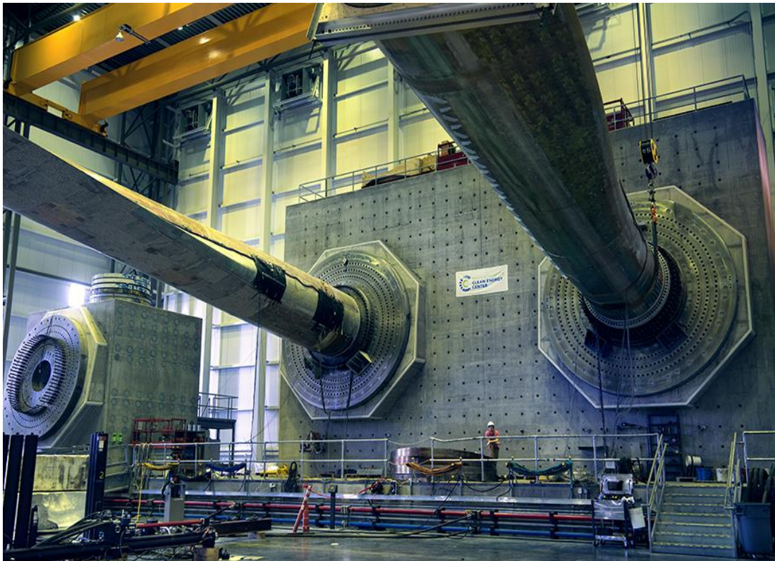
Figure 4: Existing Facility - Test Stands with Blades Affixed
