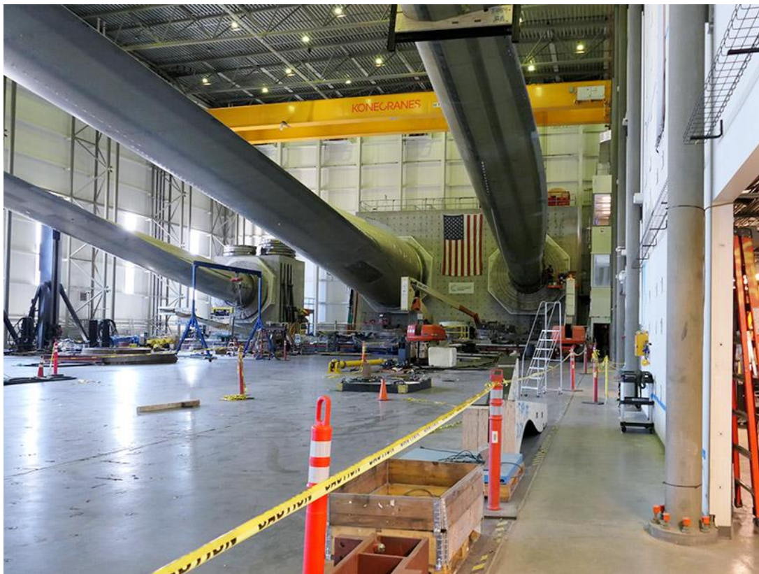
Figure 2: Existing Facility - Blades Affixed to Test Stands
