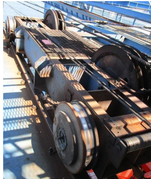
Photo above shows crane hoist trolley, trolley wheels, and trolley rail.
