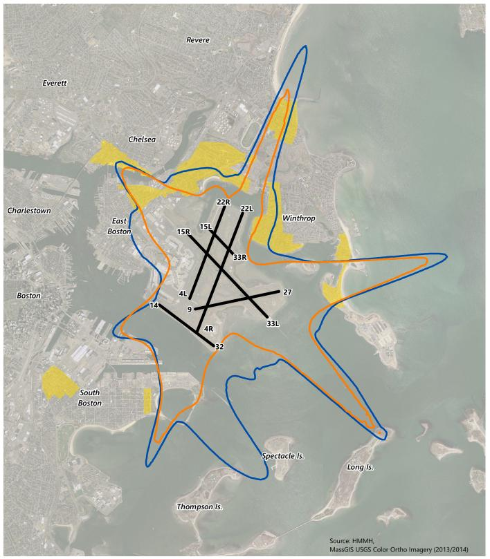
FIGURE 6-12 Comparison between 2016 (INM 7.0d) and 2016 (AEDT 2c) DNL 65 dB Contours
