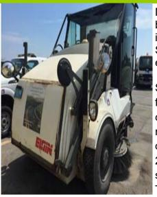
Massport's Fleet Maintenance has been using a bio-based hydraulic fluid in street sweepers serving Logan Airport. Three Elgin Pelican Street Sweepers have been piloting a program on the effectiveness of using a bio-based hydraulic fluid.
