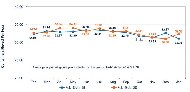
Productivity is determined by averaging the number of containers lifted per hour per crane during the time vessel operations are underway. Vessel operation time is determined by the time the vessel is at berth minus delays.
