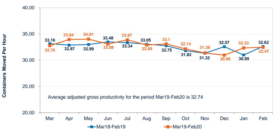
Productivity is determined by averaging the number of containers lifted per hour per crane during the time vessel operations are underway. Vessel operation time is determined by the time the vessel is at berth minus delays.
