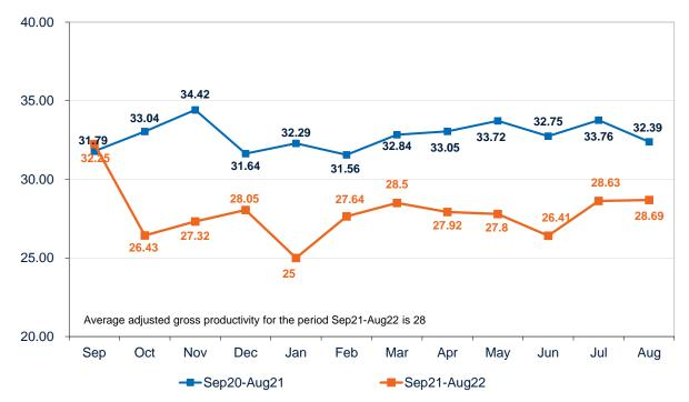
Productivity is determined by averaging the number of containers lifted per hour per crane during the time vessel operations are underway. Vessel operation time is determined by the time the vessel is at berth minus delays.
