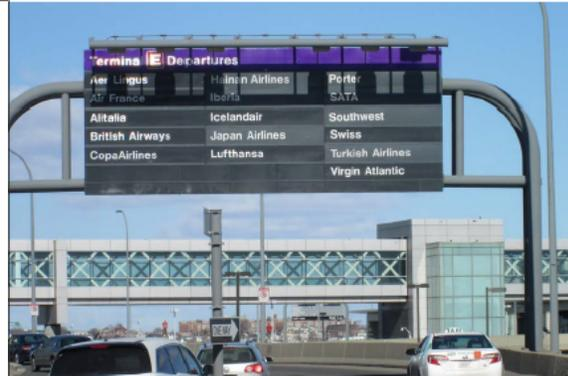
Resolution refers to the number of pixels in a given area. Pixel pitch is the distance from the center of an LED pixel to the center of the next LED pixel and it is measured in millimeters. Resolution is measured in pixel pitch for LED signs. Lower resolutions create larger characters which are viewable at farther distances, while higher resolutions allow for sharper characters. The tighter the pixel pitch the more costly the sign, therefore finding the balance is important.
